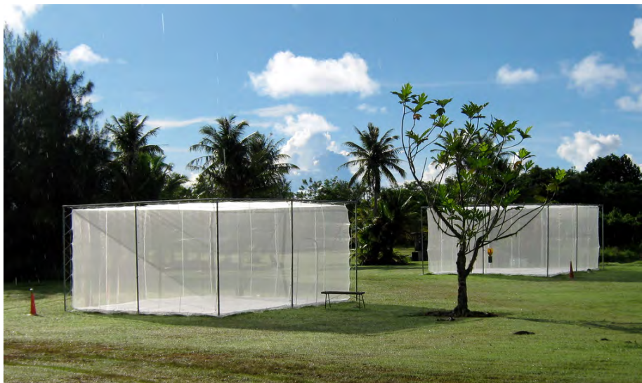
Figure 6: Large field cages for testing SPLAT-RB attracticide.
